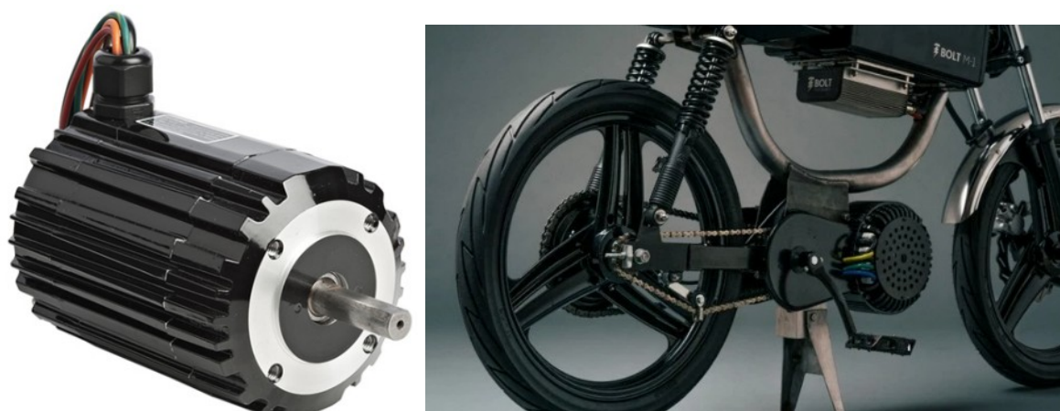
Fig. 1.1.3 In runner BLDC motor mounted on a moped
