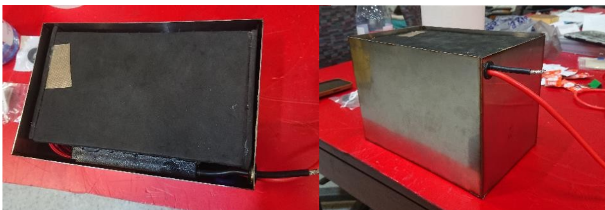
Fig. 4.3.7 Battery housing made of steel
