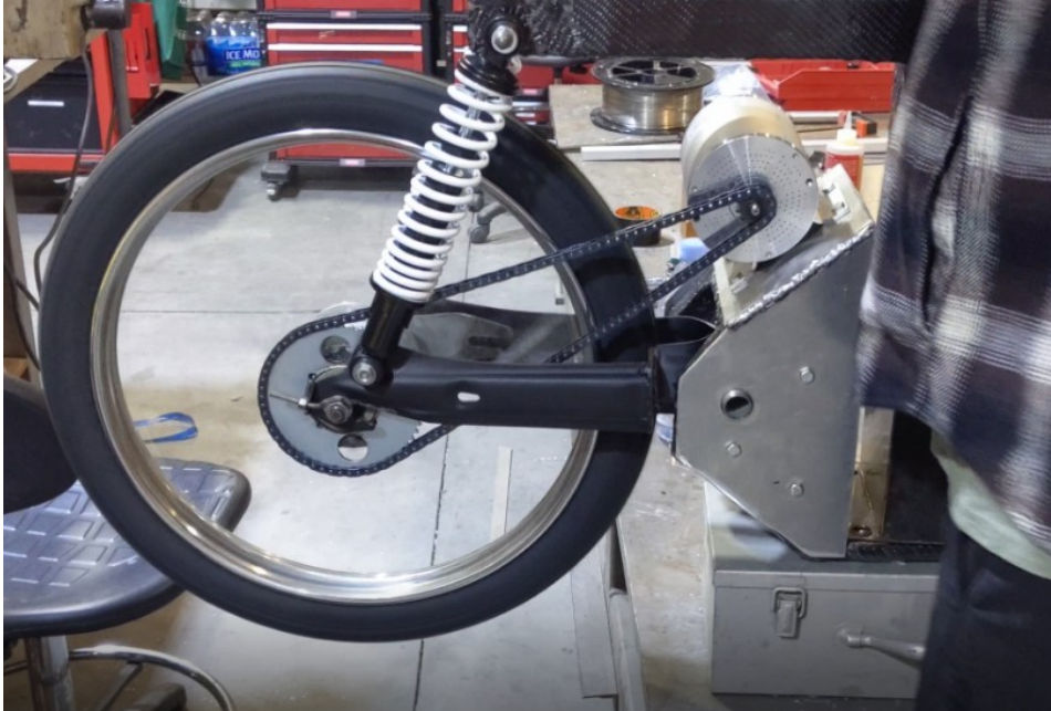
Fig. 5.3.10 Motor testing with reinforced frame
