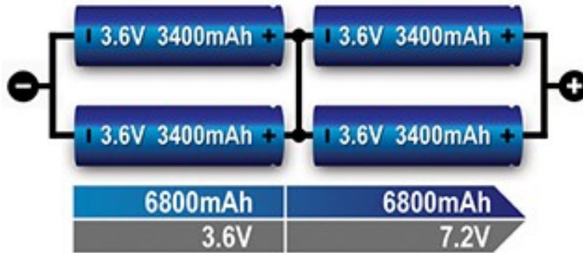
Fig. 4.2.8 Battery connection diagram in series and parallel
