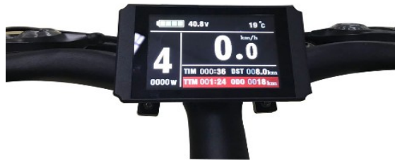
Fig. 1.4.3 Example of a standard ebike display
