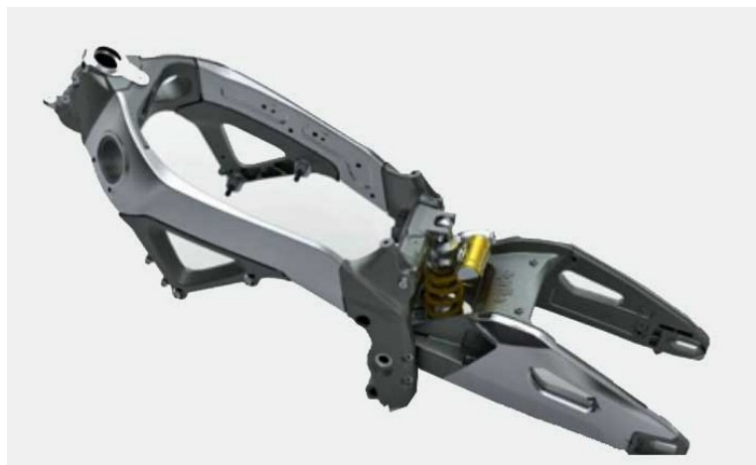
Fig. 2.3.4 Example of a perimeter frame
