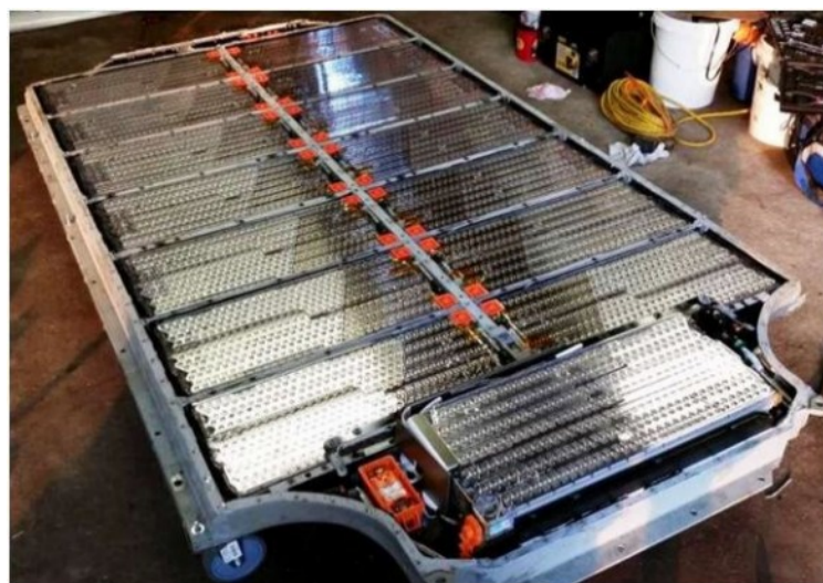
Fig. 4.2.5 Picture of a battery from a "Tesla" car
