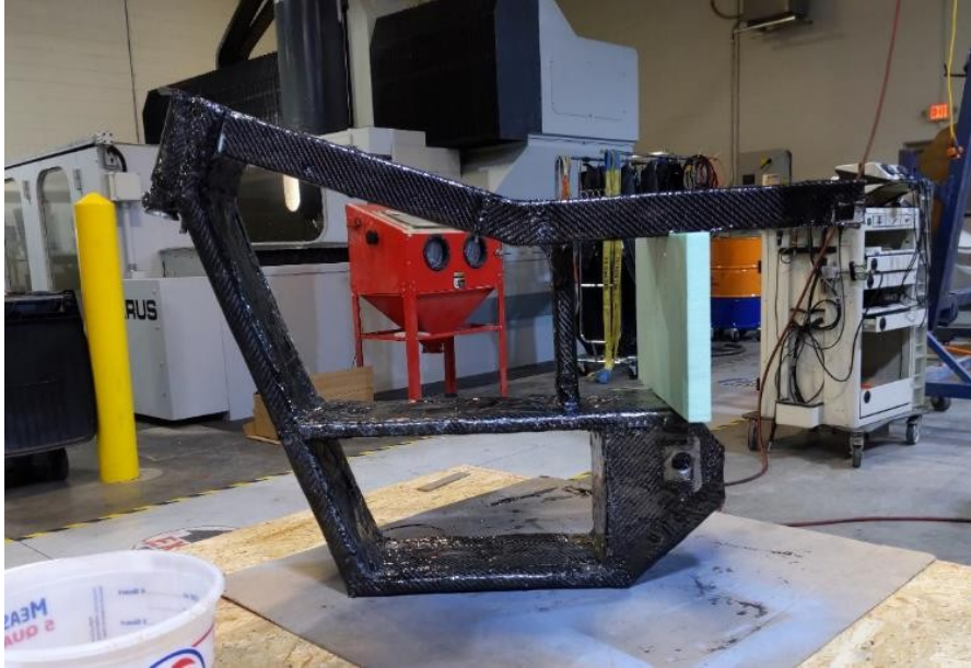
Fig. 5.3.8 Complete frame wrapped in carbon fiber
