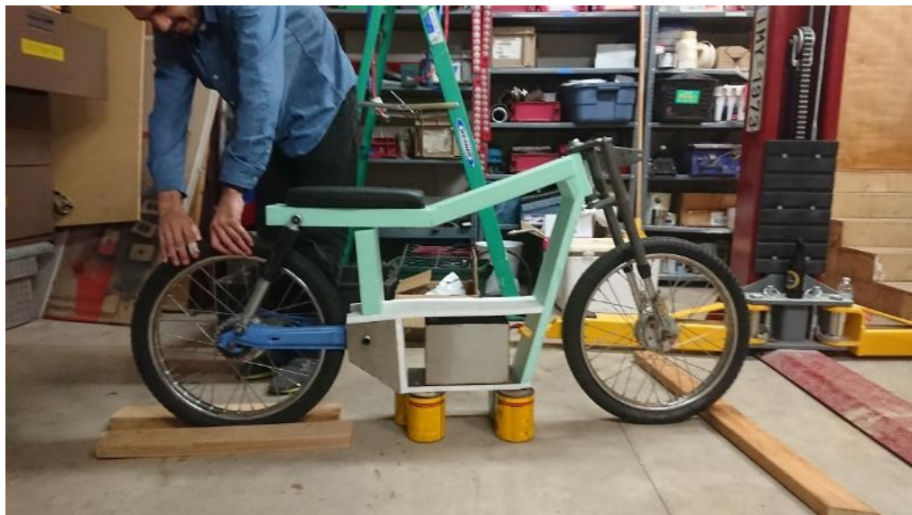
Fig. 5.3.3 Checking the fit of the parts in the frame
