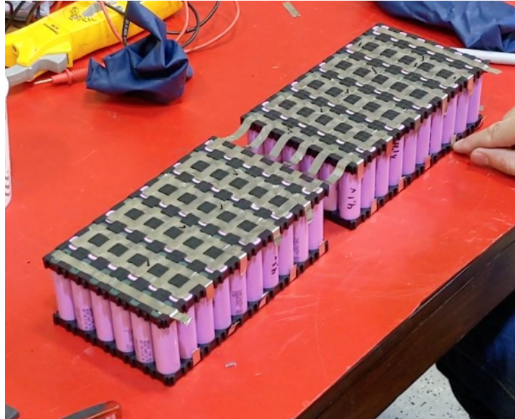
Fig. 4.3.2 The picture with the main connections made on the battery
