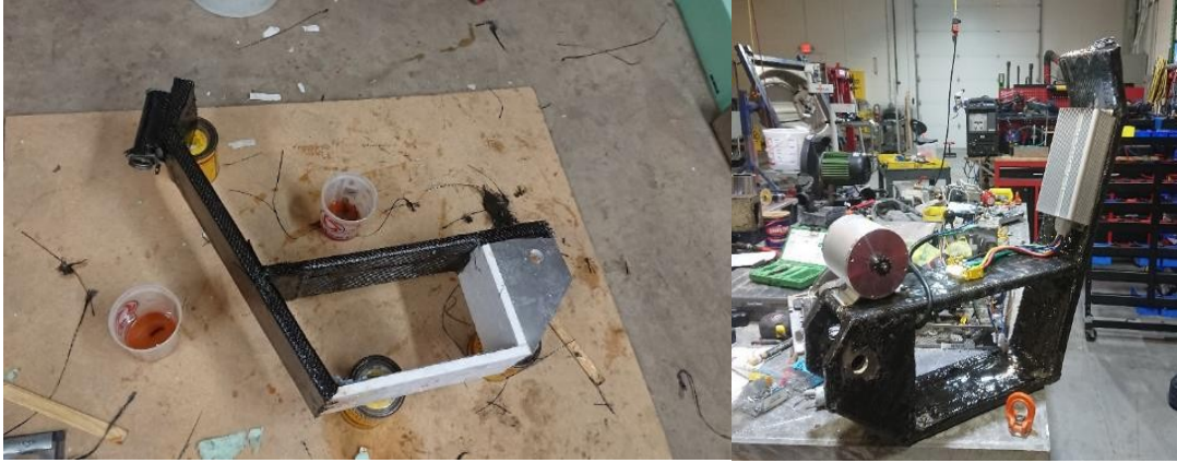
Fig. 5.3.4 Bottom frame wrapped with carbon fiber
