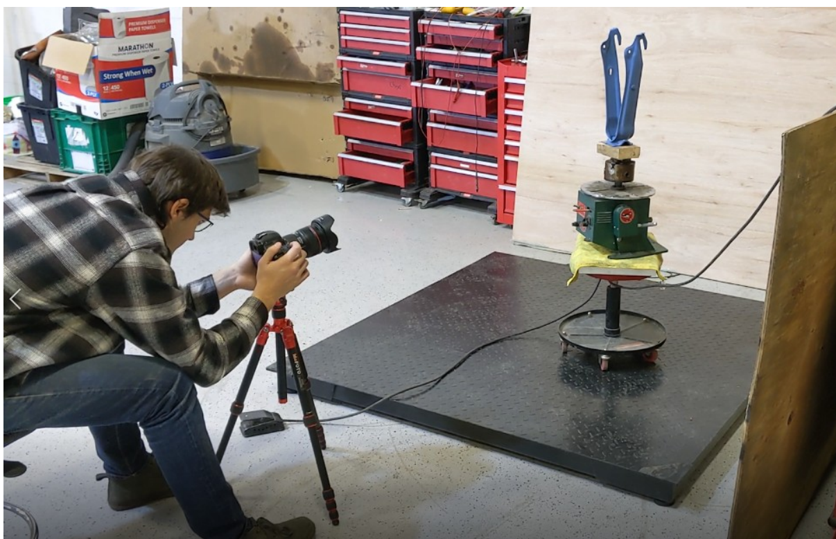
Fig. 3.2.1 taking photos of the rear subframe to be used with photogrammetry
