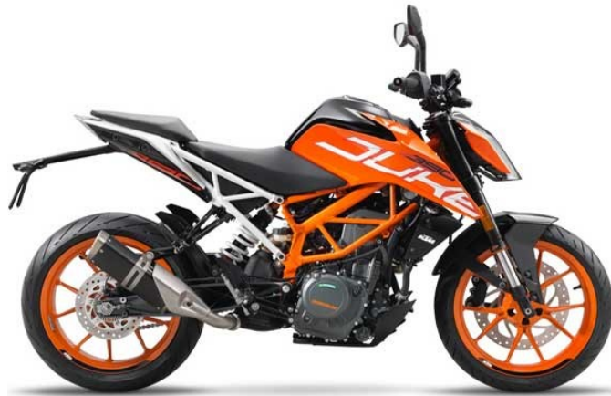
Fig. 2.3.5 „KTM 390 Duke” (Utilizes a trellis frame)
