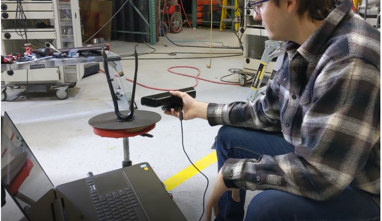
Fig. 3.2.2 3d scanning using the „Xbox Kinect”
