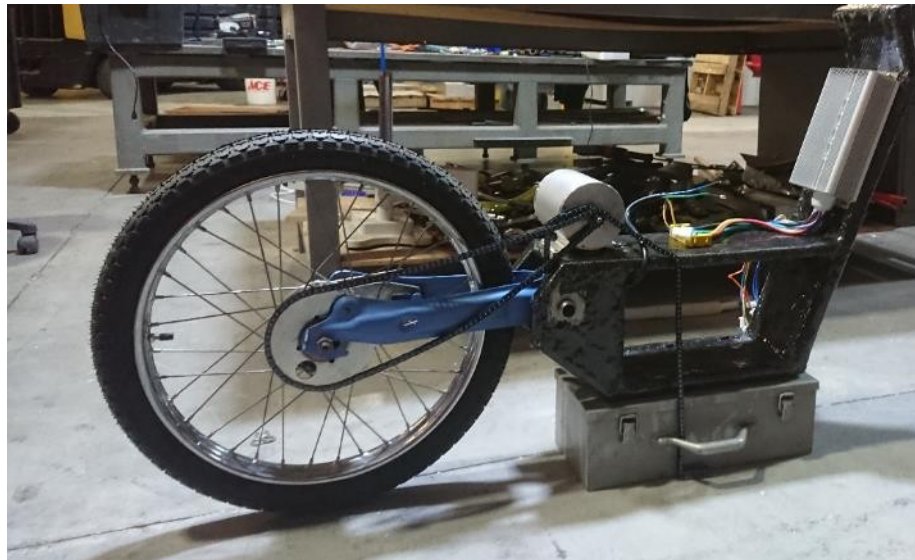
Fig. 5.3.5 Problem with rear chain rubbing on rear trailing arm
